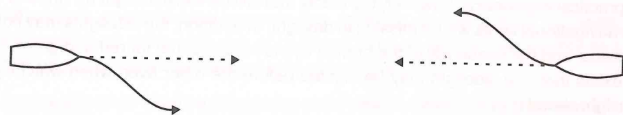
A typical head-on situation, two power driven vessels on reciprocal courses. Both alter their course to starboard
