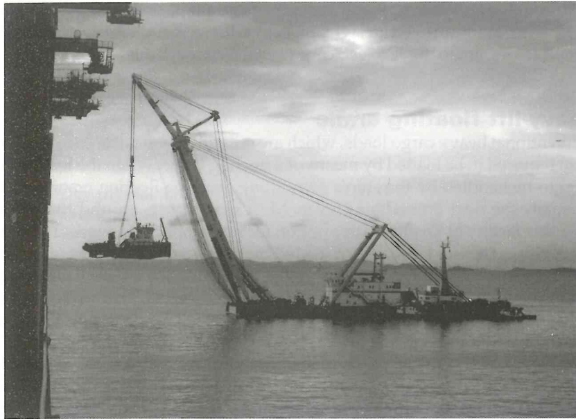
Fig. 2.24 The Smit 'Cyclone' floating shear leg barge, engages in a general cargo heavy-lift operation on the vessels offshore side.
