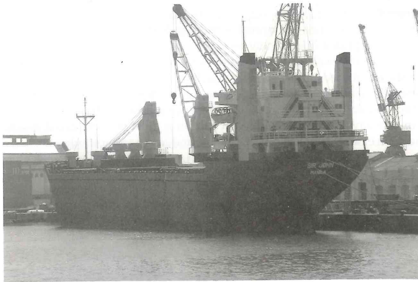
Fig. 1.12 The 'Sir John' general-purpose cargo vessel lies starboard side to in the Port of Barcelona. Fitted with two heavy-duty deck cranes both situated on the starboard side of the vessel.
