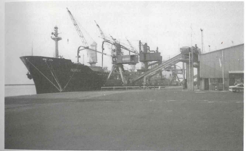
Fig. 1.14 The 'Norvik' general cargo vessel pictured in the Port of Limassol, Cyprus. The ship has turned her deck cranes outboard to allow access for the suctions of the grain elevators to discharge a bulk cargo of grain.
