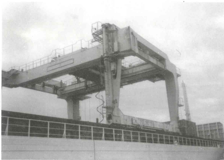
Fig. 1.17 Dominant gantry crane mounted above the deck and tracked to move fore and aft. Has an SWL of 25 tonnes and outreach extending to 35 m, either side. Single-man overhead operation
