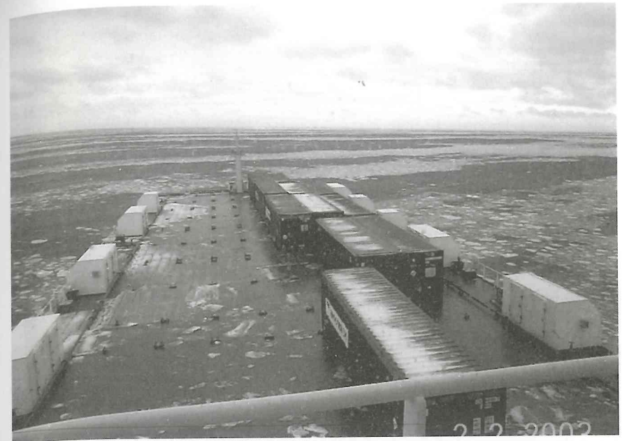
Fig. 2.25 The steel deck of the 'Baltic Eider' fitted to receive containers overall. Seen in a part-loaded condition passing through light ice in the Baltic Sea.
