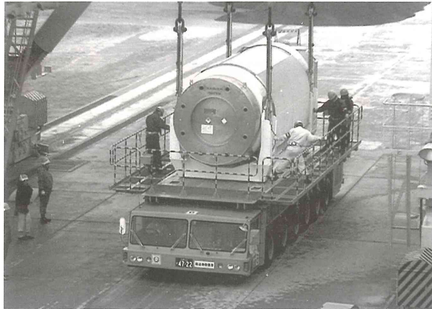
Fig. 2.16 A nuclear waste flask (weighs up to 120 tonnes) is loaded to a customized low load transporter by means of individual heavy duty straps and shackles.
