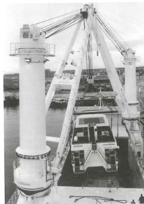
Fig. 2.14 Use of heavy duty lifting beams. Two Huisman shipboard cranes (each at 275-tonne SWL) hoist the new ferry load Fiorello, by means of two heavy-duty lifting beams, aboard the Mammoet vessel 'Transporter'.
