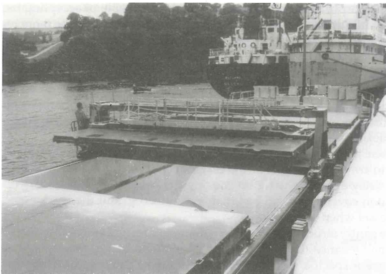
Fig. 1.16 A low lying tracked gantry crane operates down the hatch coaming to remove hatch lids from a small coasting vessel carrying bulk cargoes. Single-man operation drives the gantry in a fore and aft direction once the hatch lid is lifted clear of the hatch track.
