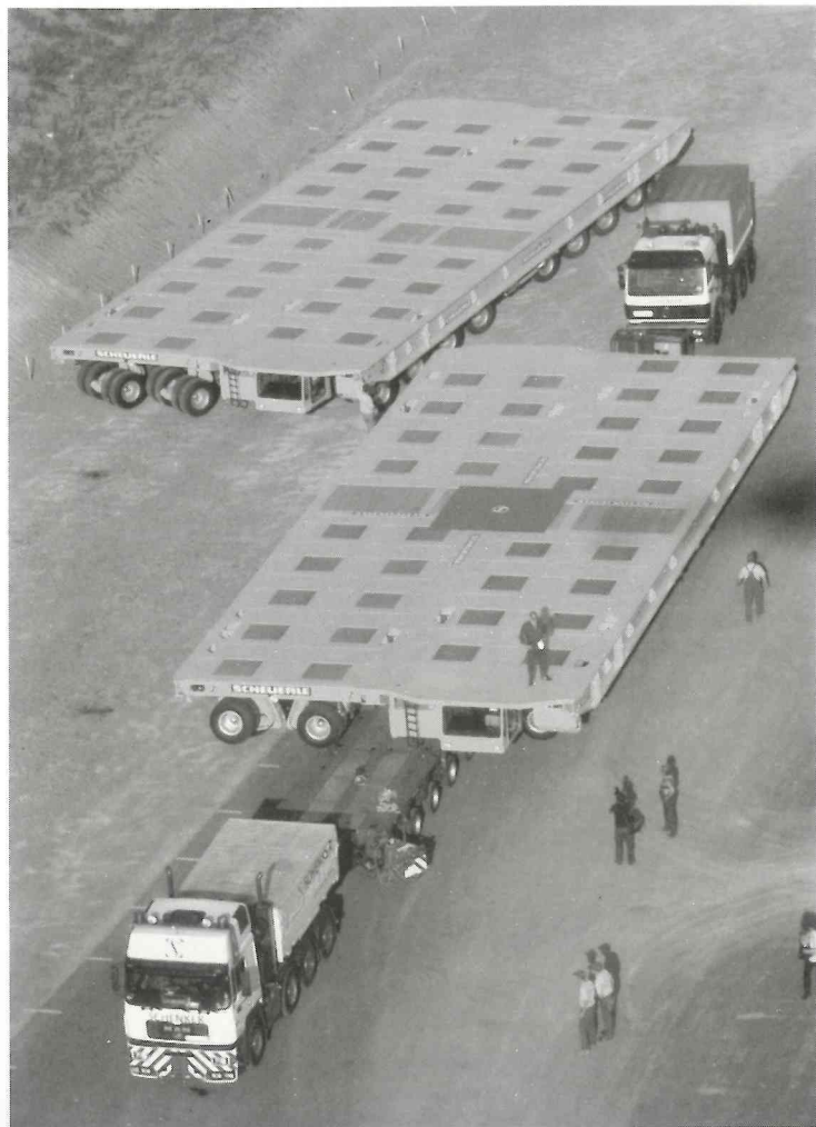
Fig. 2.31 Multi-wheel heavy load transports. Manufactured by the Scheuerle Company of Germany. The mobile platforms provide multi-axle transport for the large heavy load and are regularly inter-connected for the project load carrying up to 10 000 tonnes. Variations for smaller loads range from the 15-tonne low-bed trailers to platform trailers of up to 1000 tonnes.
