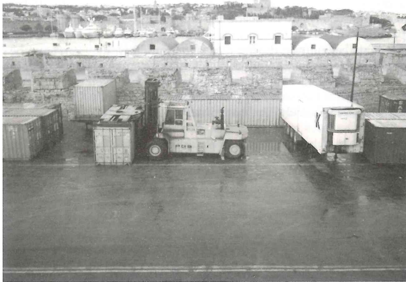
Fig. 1.23 Ground handling of large loads, like containers, can also be achieved by using the larger, high capacity 'fork lift' trucks on the quay side. Expansion forks of extended length are used for wide loads up to about 12 tonnes.
