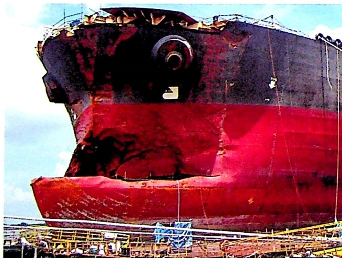
The result of human error – a damaged VLCC following a collision in the Singapore Strait
