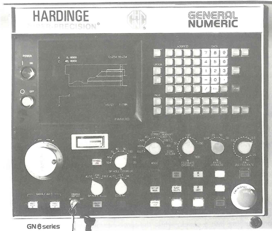
Figure 8.63 A machine controller with built-in CRT to facilitate program proving.
