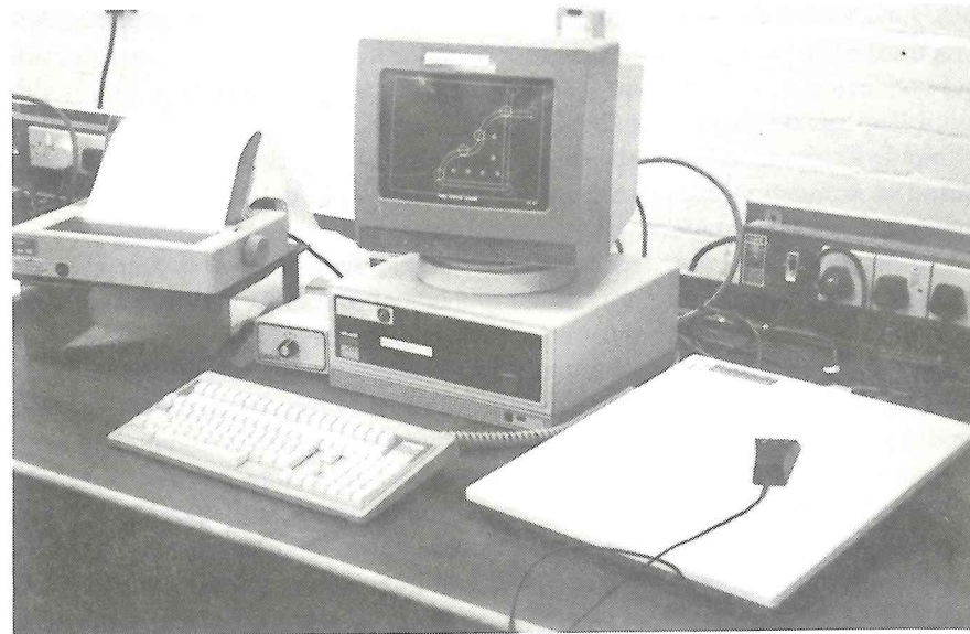
Figure 10.1 General arrangement of a CAPP work station.
