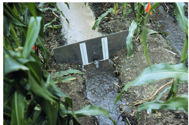
Fig. 20.12 Blocked furrow infiltrometer (Credit NRCS)
