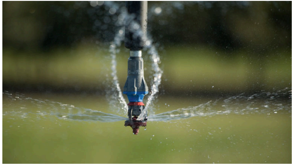
Fig. 12.8 Rotator on drop tube (Credit NRCS)
