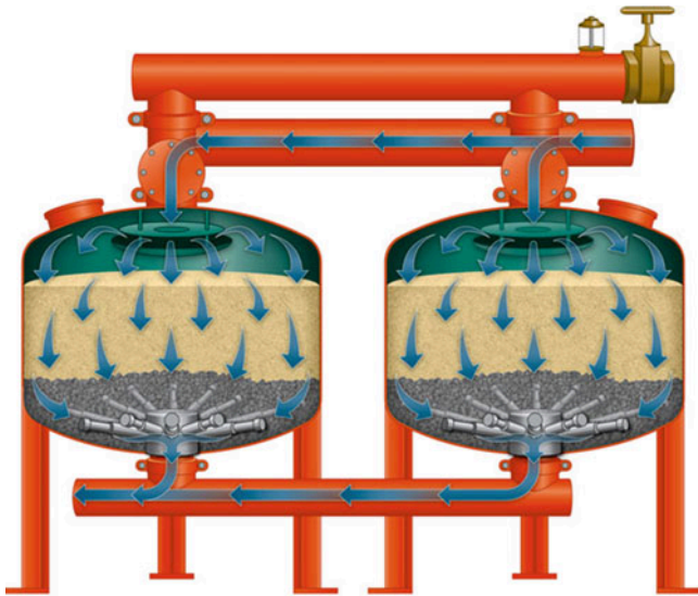
Fig. 17.5 Sand media filters (Credit Yardney Corp)
