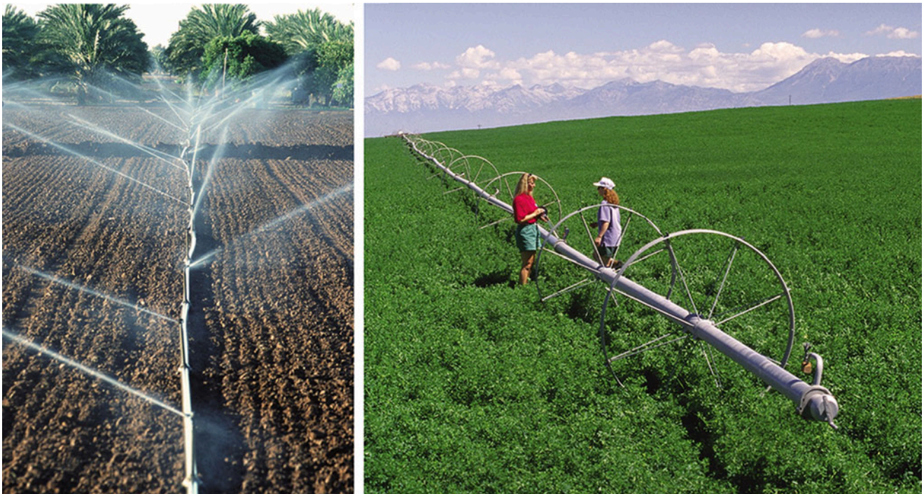
Fig. 1.10 Hand-line and wheel-line (Credit NRCS)
