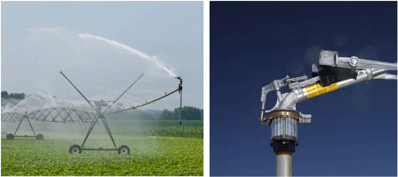
Fig. 12.4 Big gun at end of center pivot irrigation system (Credit NRCS)
