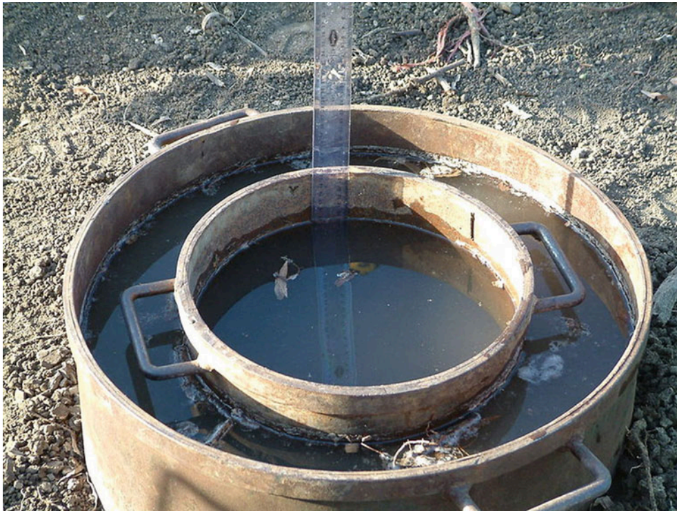
Fig. 20.8 Double ring infiltrometer
