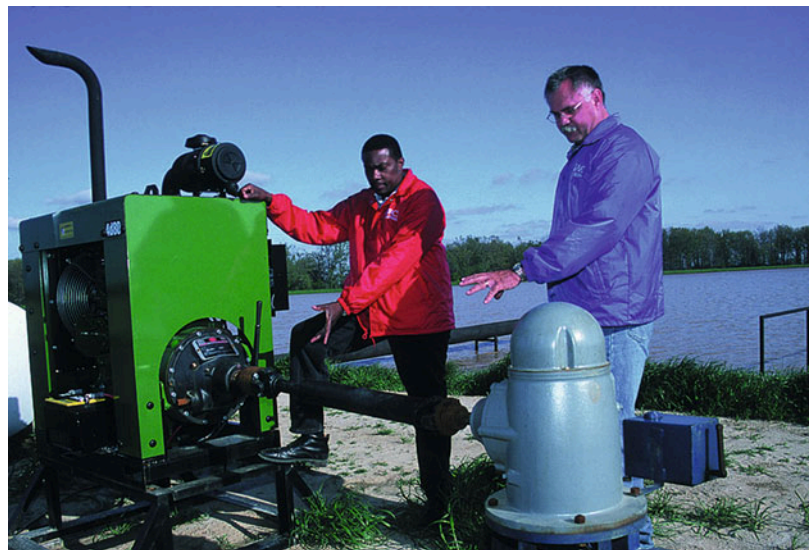
Fig. 9.2 Centrifugal pump and motor (Wikipedia)
