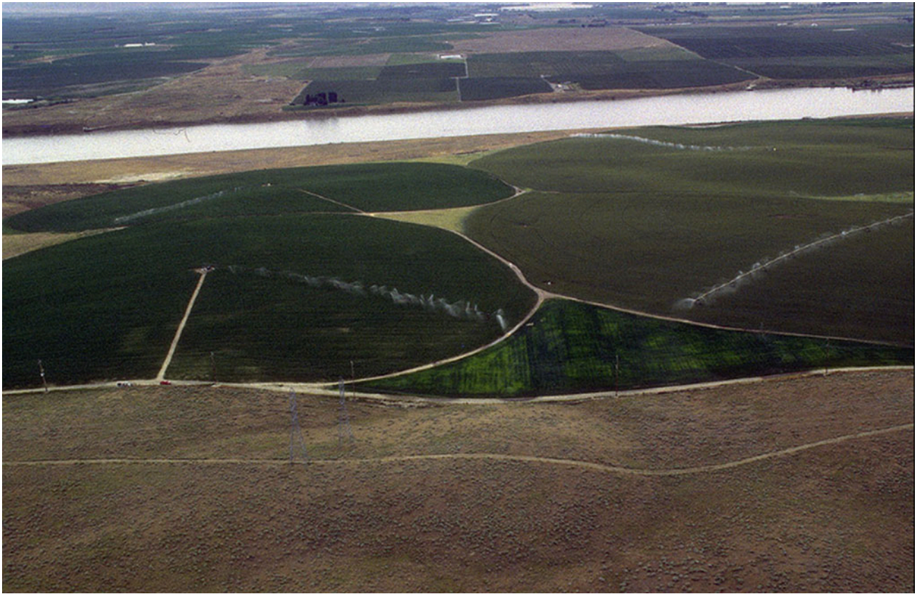
Fig. 12.1 Potato fields under irrigation with center-pivot sprinklers in Idaho, USA (Credit: US Army Corps of Engineers)
