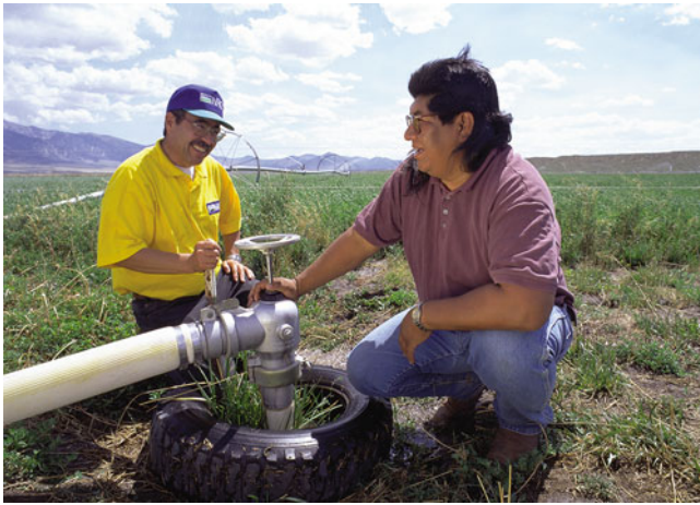
Fig. 14.3 Wheel-line or hand-line hydrant (Credit NRCS)
