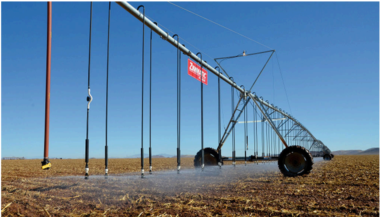
Fig. 12.6 Drop tube sprayers
