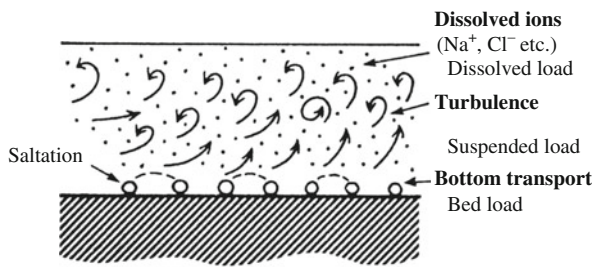
Fig. 2.8 Different forms of transport in water. Sediment grains may be carried in suspension if the vertical component of the turbulence is equal to the falling velocity of the grains. Larger grains are carried along the bottom due to the shear stress
