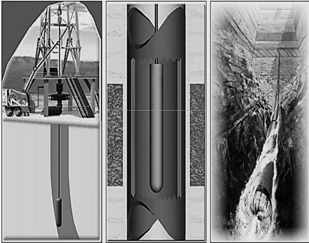
Fig. 16.4 Open hole ( left ), cased hole ( middle ) and LWD/MWD ( right ) logging techniques. Logs run in an open hole which has just been drilled but not cased. Logs run after the
