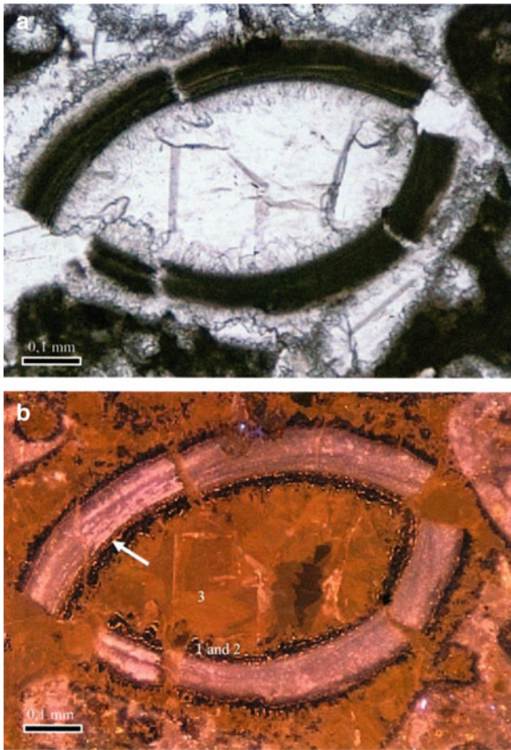
Fig. 5.54 (a) shows a well cemented limestone with an articulated ostracod in the middle. From this transmitted light view it is not possible to differentiate between the three different cement generations which are clearly visible with cathodoluminescence microscopy (b). Cement generations 1 and 2 have been precipitated before compaction of the fossil, because these cements are missing on the broken surfaces which are due to early burial compaction of the sediment. The third cement generation (3) is a post-compaction precipitation filling the remaining primary porosity and cracks in the fossil. Thin section as seen in plane polarised light and cathodoluminescence. Upper Tertiary, Iran. (Photographs courtesy of Torleiv Torgersen)
