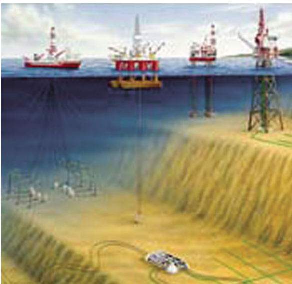
Fig. 17.18 Permanent installation of 4C cables on the sea bottom over a producing field. It improves data quality by ensuring more accurate receiver locations within the repeated 3D surveys over a period of time
