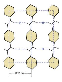
Fig. 2.35 Schematic representation of the supramolecular structure of aramid fiber, Kevlar 49. The structure consists of radially arranged, axially pleated crystalline sheets [from Dobb et al. (1980), used with permission]
