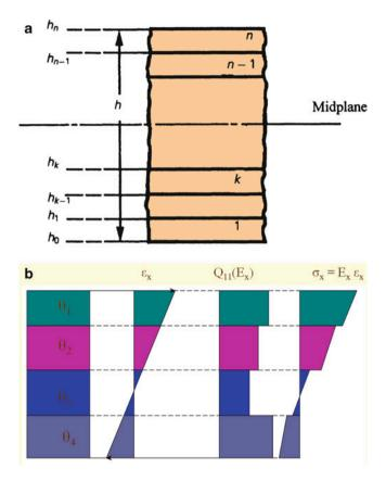
**Fig. 11.6** (a) A laminated composite made up of *n* stacked plies. (b) Variation of strain and stress through the thickness in a four-ply laminated composite
