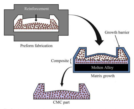
Fig. 7.4 Schematic of the directed metal oxidation process of Lanxide Corp. (Courtesy of Lanxide Corp.)
