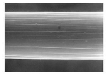
Fig. 2.20 Scanning electron micrograph of PAN-based carbon fiber (fiber diameter is 8  $\mu$ m). Note the surface markings that stem from the fiber drawing process
