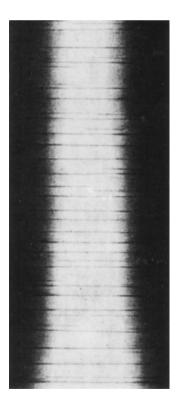
Fig. 14.3 Delaminations, as observed by contrast-enhanced X-ray radiography in a [0°/±45°/90°], carbon/epoxy laminate upon fatigue testing. [From Bergmann (1985), used with permission]
