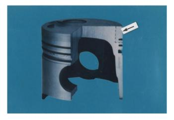
Fig. 6.27 A cutout of a squeeze cast piston with MMC inserts indicated by *dotted lines*. [Courtesy of Toyota Motor Co.]
