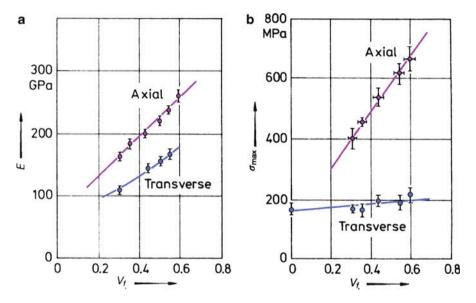
Fig. 6.19 Properties of Al<sub>2</sub>O<sub>3</sub>/Al–Li composites as a function of fiber volume fraction ( $V_f$ ): (a) axial and transverse Young's modulus vs. fiber volume fraction, (b) axial and transverse ultimate tensile strength vs. fiber volume fraction. [From Champion et al. (1978), used with permission]
