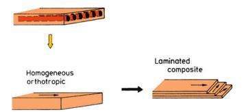
**Fig. 11.1** Macromechanical analysis of laminate composites. A unidirectional ply is treated as a homogeneous, orthotropic material. Many such plies are stacked in an appropriate order (following laminated plate or shell theory) to make the composite [reprinted from McCullough (1971), courtesy of Marcel Dekker, Inc.]
