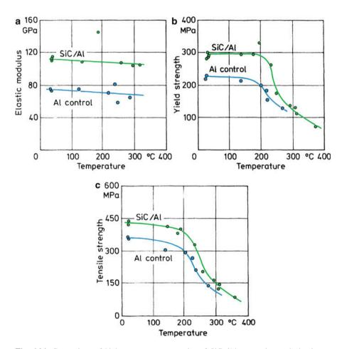
Fig. 6.24 Comparison of high-temperature properties of  $SiC_w/Al$  composites and aluminum: (a) elastic modulus, (b) yield stress, (c) ultimate tensile strength. [From Phillips (1978), used with permission]
