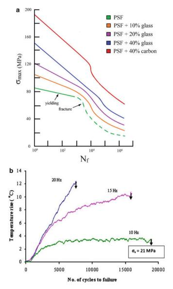
**Fig. 13.4** (a) *S–N* curves of unreinforced polysulfone (PSF) and composites with a PSF matrix and different amount of short fibers (glass and carbon) [after Mandell et al. (1983)]. (b) Temperature rise under fatigue for glass fiber/polypropylene composites (Goel et al. 2009). At a given stress amplitude, temperature rises more quickly at higher frequency and leads to premature failure of the composite
