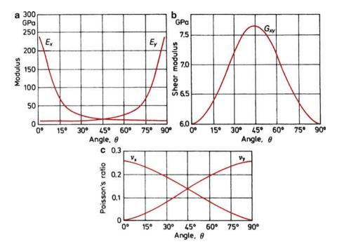
Fig. 11.4 Variation of elastic constants with fiber orientation angle for a 50 v/o carbon/epoxy composite: (a) longitudinal and transverse Young's moduli ( $E_x$  and  $E_y$ ), (b) shear modulus ( $G_{xy}$ ), and (c) Poisson's ratio ( $v_x$  and  $v_y$ )
