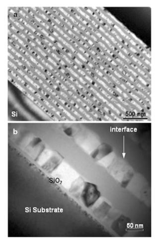
**Fig. 15.5** (a) Microstructure of SiC/Al nanolaminate. (b) TEM micrography shows the well-bonded interface and absence of any reaction product at the interface. SiO<sub>2</sub> forms on the surface of SiC
