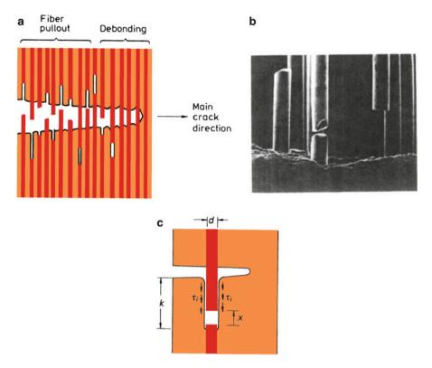
**Fig. 12.4** (a) Schematic of fiber pullout in a continuous fiber composite. (b) Fiber pullout in a B/Al system. (c) Schematic of an isolated fiber pullout through a distance x against an interfacial shear stress,  $\tau_i$
