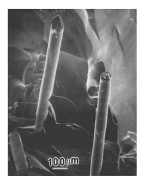
boundaries and is, therefore, very smooth (Venkatesh and Chawla 1992). Crack deflection at the interface leads to fiber pullout etc., which contribute to toughness (see also Chap. 10). For detailed analysis of this important topic of interface engineering for toughness, the reader is referred to a review by Chawla et al. (2000).
