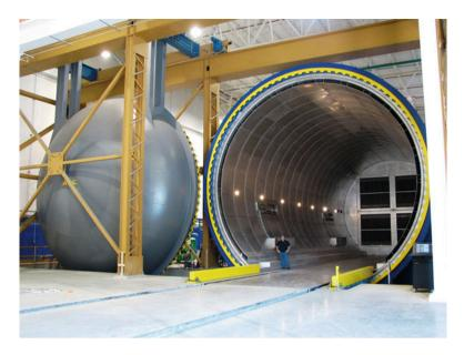
**Fig. 5.6** A large autoclave that is used to make the wings of Boeing 787. An idea of the size of the autoclave can be had from the height of the person standing inside the autoclave (courtesy of ASC Process Systems Inc., Sylmar, California)
