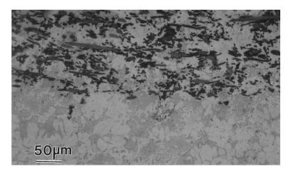
**Fig. 6.28** Microstructure of the cylinder liner showing the unreinforced Al alloy (*bottom*) and fiber (alumina + carbon)-reinforced (*top*) portions
