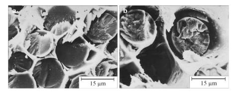
**Fig. 6.25** Tensile fracture in Nicalon fiber/aluminum: (a) at room temperature showing a planar fracture, (b) at 500 °C showing fiber/matrix separation and fiber pullout leaving a hole. [Courtesy of K. Okamura]
