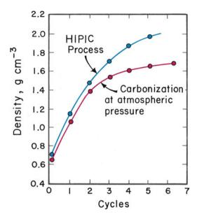
treatment. For the fabrication of C/C composites, up to a density of 1.4 g/cm<sup>3</sup>, atmospheric processing and HIPIC have about the same efficiency. For density values greater than 1.4 g/cm<sup>3</sup>, HIPIC shows much better efficiency than processing at atmospheric pressure.
