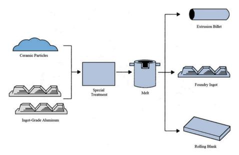
Fig. 6.2 Schematic of the Duralcan process
