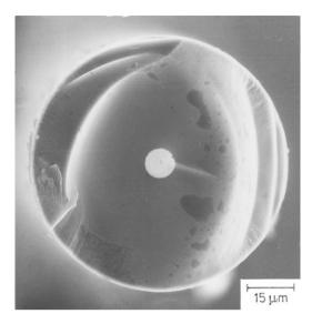
strength of boron. The average tensile strength of boron fiber is 3–4 GPa, while its Young's modulus is between 380 and 400 GPa.
