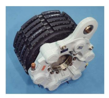
Fig. 8.8 A carbon/carbon brake assembly that is used on a Boeing 767 airplane (courtesy of Alied-Signal Corp.)
