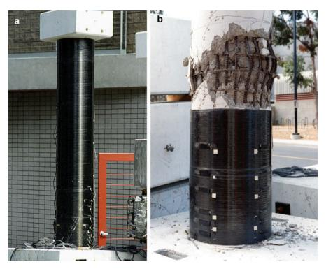
**Fig. 5.29** (a) A concrete column wrapped around with a jacket of carbon fiber/epoxy composite while (b) on application of a compressive load, spalling of concrete and buckling of the steel reinforcement bars can be seen in the part of the concrete column without the composite jacket. In the portion of the column protected with a composite jacket, there is no visible effect (courtesy of B. Kad.)
