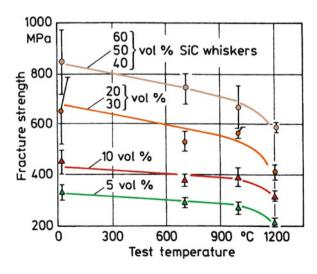
Fig. 7.21 Toughness gains are obtained by incorparating SiC whiskers in alumina [Tiegs and Becher (1986), used with permission]
