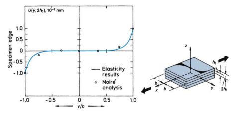
**Fig. 11.11** Surface displacements of a symmetric angle-ply laminate subjected to axial tension. Experimental data points were determined by the Moiré technique [from Pipes and Daniel (1971), used with permission]
