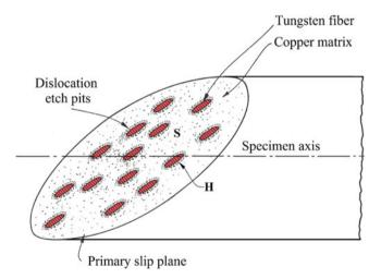
**Fig. 6.16** A primary plane section of a metal matrix composite is shown as having a hard zone (high dislocation density) around each fiber and a soft zone (low dislocation density) away from the fiber
