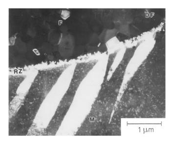
**Fig. 6.14** A controlled amount of interfacial reaction at the  $Al_2O_3$  fiber/Mg alloy matrix interface. M, F, and RZ denote matrix, fiber, and reaction zone, respectively. Dark field (DF) transmission electron micrograph
