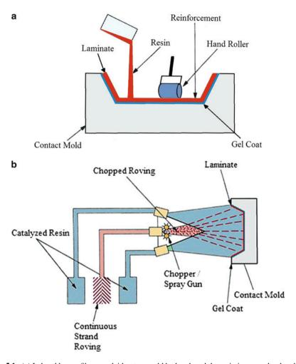
$\begin{tabular}{ll} Fig. 5.1 & (a) In hand layup, fibers are laid onto a mold by hand, and the resin is sprayed or brushed on. (b) In spray-up, resin and fibers (chopped) are sprayed together onto the mold surface $ (a) $ (b) $ (b) $ (b) $ (c) $ (c)$
