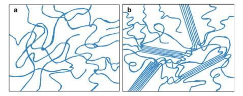
Fig. 3.3 Possible arrangements of polymer molecules: (a) amorphous, (b) semicrystalline
