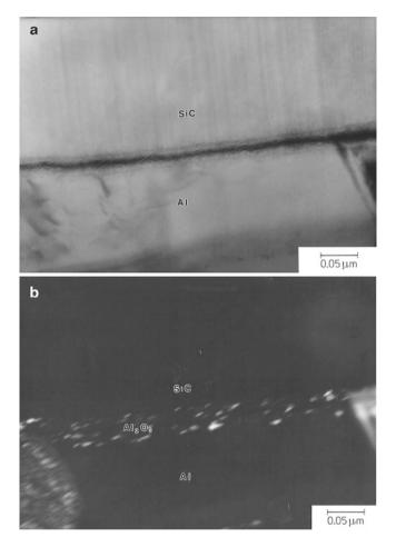
Fig. 6.18 Interface in  $SiC_w/Al$  composite: (a) bright field TEM, (b) dark field TEM showing the presence of  $A1_2O_3$  at the interface. [From Fu et al. (1986), ©ASTM, reprinted with permission]
