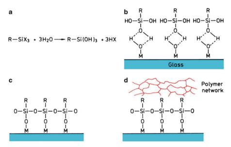
**Fig. 5.11** Chemical bridge theory of a silane coupling agent: (a) hydrolysis of silane to silanol; (b) hydrogen bonding between hydroxy groups of silanol and a glass surface; (c) polysiloxane bonded to a glass surface; and (d) resin-compatible functional groups *R* form part of the polymer matrix [from Hull (1981), reprinted with permission]
