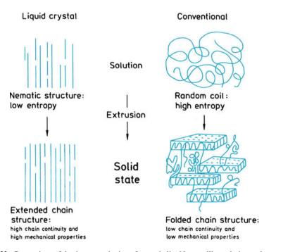
**Fig. 2.32** Comparison of dry jet—wet spinning of nematic liquid crystalline solution and conventional spinning of a polymer [reprinted from Jaffe and Jones (1985), p 349, courtesy of Marcel Dekker, Inc.]
