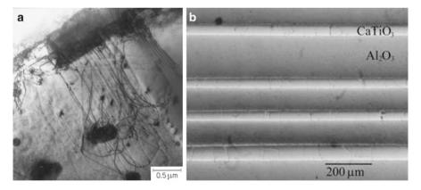
**Fig. 10.11** (a) Dislocations generated at SiC whiskers in an aluminum matrix in an in situ thermal cycling experiment done in a high-voltage electron microscope [from Vogelsang et al. (1986), used with permission]. (b) Cracking in the CaTiO<sub>3</sub> layer in a CaTiO<sub>3</sub>/Al<sub>2</sub>O<sub>3</sub> composite due to thermal stresses generated during cool down from the processing temperature (from Gladysz and Chawla 2001)
