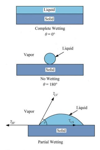
Fig. 4.1 Three different conditions of wetting: complete wetting, no wetting, and partial wetting
