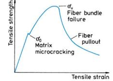
Fig. 7.12 Stress-strain curve of an aligned CMC in the longitudinal direction showing a damage-tolerant behavior
