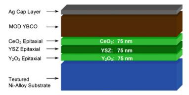
**Fig. 9.13** A schematic of final composite superconducting tape obtained by the RABiTS process. The series of buffer layers and the YBCO superconductor are deposited epitaxially on the substrate. The buffer layers transfer the texture of the metal substrate to the superconductor and prevent any reaction between the substrate and the superconductor
