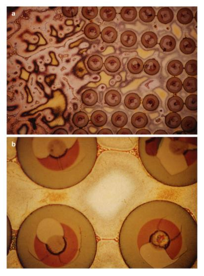
**Fig. 6.21** Transverse section of an SCS-2 SiC fiber in an Al-4.5 % Cu matrix. (a) Note the difference in the dendritic structure of the unreinforced and the fiber-rich regions of the matrix. (b) the second phase appears preferentially at the fiber/matrix interface or in the narrow interfiber region. The fiber diameter is 142  $\mu$ m in both (a) and (b). [Reprinted with permission from J Metals 37(6):45, 47, and 48, a publication of the Metallurgical Society, Warrendale, Pennsylvania]
