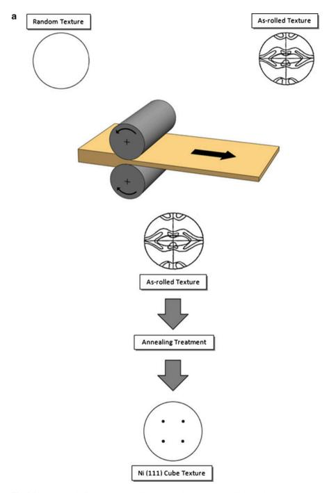
**Fig. 9.12** The RABiTS process. A metallic substrate is prepared by rolling and heat treatments to serve as a structural template for the superconducting YBCO layer, which has substantially fewer weak links than the substrate. The *circles* show the pole figures showing the specific type of grain texture obtained. (a) Cube texture in Ni (b) Final superconducting tape on Ni
