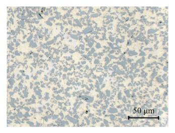
Fig. 6.6 Microstructure of a centrifugally cast WC/bronze composite
