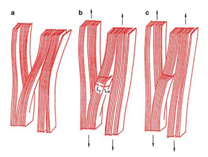
**Fig. 2.23** Model for tensile failure of carbon fiber: (a) a misoriented crystallite linking two crystallites parallel to the fiber axis, (b) basal plane rupture under the action of applied stress, (c) complete failure of the misoriented crystallite [from Bennett et al. (1983), used with permission]
