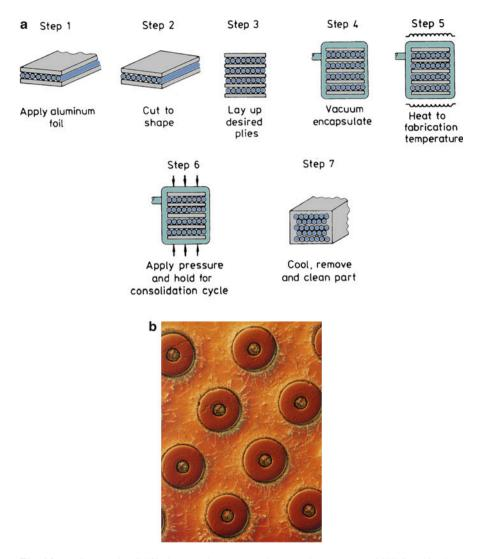
Fig. 6.8 (a) Schematic of diffusion bonding process. (b) The microstructure of SiC fiber/titanium matrix composite made by diffusion. Each fiber is  $142~\mu m$  in diameter. [Courtesy of J. Baughman]
