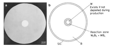
Fig. 2.10 (a) Cross-section of a 100-µm-diameter boron fiber. (b) Schematic of the cross-section of a boron fiber with SiC barrier layer
