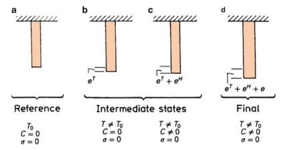
**Fig. 10.8** (a) Strain-free reference state; (b) thermal strain  $(e^T)$ ; (c) hygral  $(e^H)$  and thermal  $(e^T)$  strains; and (d) final state: hygral  $(e^H)$ , thermal  $(e^T)$ , and mechanical strain
