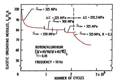
Fig. 13.8 Response of a boron fiber/aluminum matrix composite subjected to a constant cyclic stress range (225 MPa) with varying values of  $S_{\text{max}}$ , the maximum stress [after Johnson (1988)]
