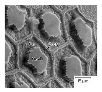
Fig. 9.7 Scanning electron microscope picture of Nb-Ti/Cu superconductor
