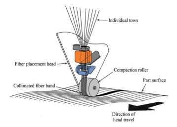
Fig. 5.4 Schematic of automatic fiber placement process
