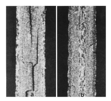
**Fig. 14.4** Comparison of crack patterns at the free edges of a carbon/epoxy laminate: (a)  $[0^{\circ}/\pm 45^{\circ}/90^{\circ}]_s$ , (b)  $[90^{\circ}/\pm 45^{\circ}/0^{\circ}]_s$ . Note the greater severity of edge delaminations in (a) than in (b). [From Bergmann (1985), used with permission]
