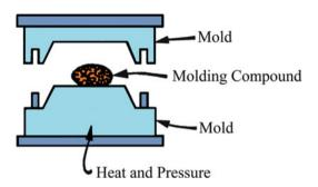
Fig. 5.10 Schematic of SMC processing
