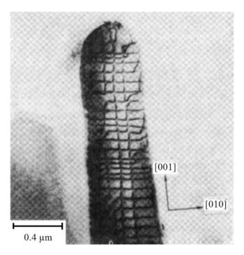
**Fig. 6.10** A network of dislocations between the NiAl matrix and a chromium rod in a unidirectionally solidified NiAl–Cr eutectic. [Reprinted with permission from Acta Mater, 19, H.E. Cline et al. 1971, Pergamon Press Ltd.]
