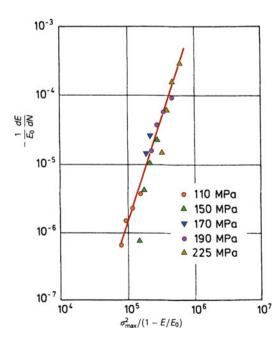
Fig. 13.13 Modulus reduction rate vs. a parameter involving the peak stress [after Ogin et al. (1985)]
