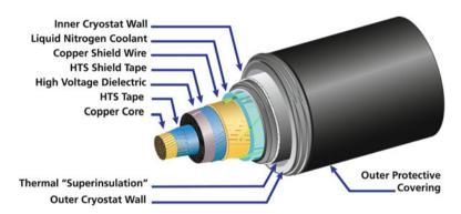
**Fig. 9.14** A schematic of a 2G superconducting cable, trade name Amperium. Note the number of different materials used (courtesy of American Superconductor Co.)
