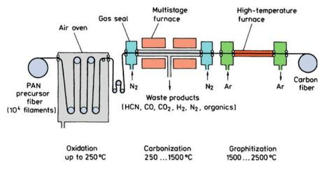
Fig. 2.15 Schematic of PAN-based carbon fiber production [reprinted with permission from Baker (1983)]
