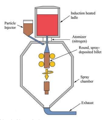
Fig. 6.7 Schematic of the spray forming process
