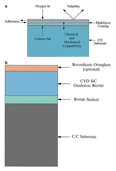
**Fig. 8.4** (a) Critical factors that should be taken into account for an oxidation protection system for carbon/carbon composites (after Strife and Sheehan 1988). (b) Schematic of a typical multi-layer oxidation protection system on a C/C substrate
