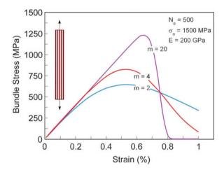
Fig. 12.9 Fiber bundle strength vs. strain in a CMC for different Weibull modulus values (courtesy of E. Lara-Curzio)
