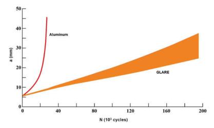
Fig. 15.8 Fatigue crack growth of GLARE compared to monolithic aluminum alloy
