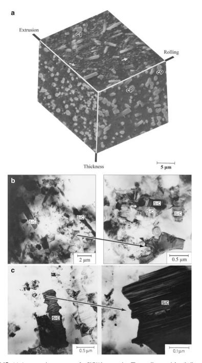
**Fig. 6.17** (a) A perspective montage of a SiC/Al composite. The smallest particles (indicated by arrows on the top face) are precipitates from the matrix as a result of aging. Silicon carbide whiskers are
