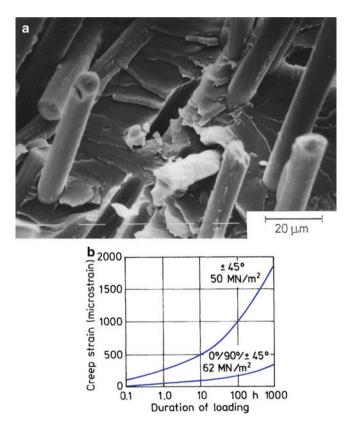
Fig. 5.20 (a) Brittle matrix fracture and fiber pullout in a short glass fiber reinforced polyethylene terephthalate (PET) composite fractured at  $-80\,^{\circ}$ C [from Friedrich (1985), used with permission] (b) Creep strains at ambient temperature for a  $\pm 45\,^{\circ}$  and for a  $0\,^{\circ}/90\,^{\circ}/\pm 45\,^{\circ}$  carbon/epoxy laminate [from Sturgeon (1978), used with permission]
