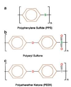
Fig. 3.10 Chemical structure of (a) PPS, (b) polyaryl sulfone, and (c) polyetherether ketone (PEEK)
