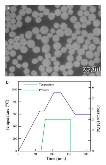
**Fig. 7.2** (a) An optical micrograph of a transverse section of a unidirectional Nicalon fiber/glass matrix composite. (b) Pressure and temperature schedule used during hot pressing of a typical composite
