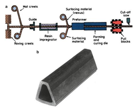
Fig. 5.3 (a) Schematic of the pultrusion process (courtesy of Morrison Molded Fiber Glass Co.). (b) A helicopter windshield post made of carbon fibers/vinyl ester resin by pultrusion. The post is 1.5 m long (courtesy of Morrison Molded Fiber Glass Co.)
