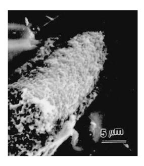
Fig. 7.26 Fracture surface single crystal alumina fiber/SnO<sub>2</sub>/glass composite showing fiber pullout. This fiber is single crystal alumina, which has no grain boundaries and is, therefore, very smooth. Crack deflection at the interface leads to fiber pullout
