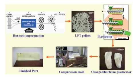
**Fig. 5.9** Extrusion/compression molding process for making long fiber reinforced thermoplastic (LFT) composites. Hot melt impregnation of fibers is used to produce tapes, rods or long pellets of LFT. Pelletized LFT material is fed into an extruder or plasticator. Plasticized LFT charge is compression molded to different product forms
