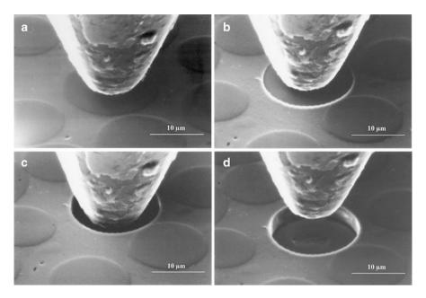
Fig. 4.10 An example of fiber pushin is shown in a series of four photographs. (a) Indenter approaching the fiber (b) touching the fiber (c) fiber pushin (d) lifting of indent (courtesy of J. Janczak-Rusch and L. Rohr)
