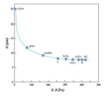
Fig. 2.2 Fiber diameter of different materials with flexibility equal to that of a nylon fiber of diameter equal to  $25 \mu m$ . Note that one can make very flexible fibers out of brittle materials such as glass, silicon carbide, alumina, etc., provided one can process them into a small diameter
