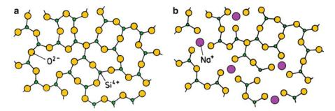
Fig. 2.6 Amorphous structure of glass: (a) a two-dimensional representation of silica glass network and (b) a modified network that results when  $Na_2O$  is added to (a). Note that  $Na^+$  is ionically linked with  $O^{2-}$  but does not join the network directly
