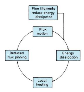
**Fig. 9.2** Flux movement in a superconductor is caused by any change in current or field
