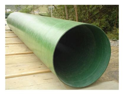
$\textbf{Fig. 5.24} \ \ A \ \ \text{filament wound pipe (diameter} = 2 \ m) \ \ \text{made for irrigation purposes in Ecuador.}$  (courtesy of Odebrecht Co.)
