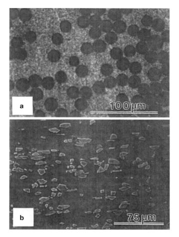
**Fig. 6.1** (a) Transverse cross-section of continuous alumina fiber/magnesium alloy composite. (b) Typical microstructure of a silicon carbide particle/aluminum alloy composite. Note the angular nature of SiC particles and alignment of particles along the long axis
