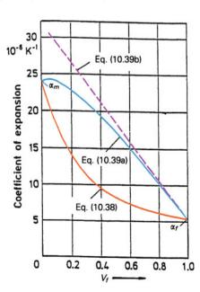
Fig. 10.7 Longitudinal and transverse linear thermal expansion coefficients vs. fiber volume fraction for alumina fiber in an aluminum matrix
