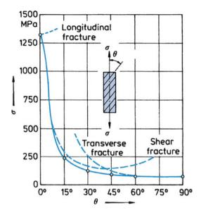
**Fig. 12.14** Variation of strength with fiber orientation for boron/epoxy. Quadratic interaction criterion (*solid curve*) shows better agreement with experimental data than the maximum stress criterion (*dashed curve*) [after Pipes and Cole (1973)]
