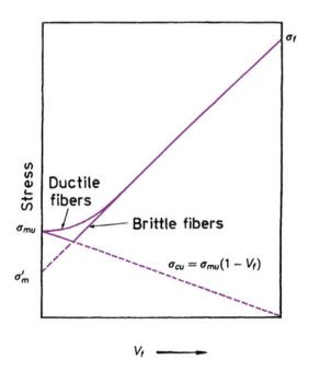
Fig. 12.2 Strength of the composite vs. fiber volume fraction for a composite with matrix having a greater strain at fracture than the fiber. Single fracture occurs to the left of cross-over point, multiple fracture occurs to the right
