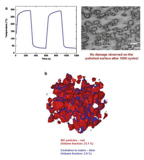
Fig. 13.15 (a) Surface of  $SiC_p/Al$  composite after thermal cycling. No damage is visible on the surface. (b) Same sample examined by X-ray tomography shows damage in the interior. *Blue* color shows cavitation, about 2 % by volume. The SiC particles are about 25–30  $\mu$ m in diameter and 20 vol.% [courtesy of N.C. Chapman and N. Chawla, Arizona State University]
