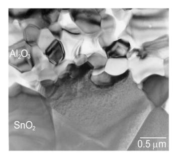
**Fig. 7.24** Roughness induced mechanical keying at the interface between alumina and SnO<sub>2</sub>. Note the tortuous nature of the interface. TEM [Gladysz et al. (1999)]
