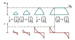
Fig. 10.17 Schematic of variation of tensile stress in a fiber  $(\sigma_f)$  and interface shear stress  $(\tau)$  with different fiber aspect ratios (l/d)
