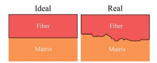
Fig. 4.2 (a) An ideal planar interface between reinforcement and matrix. (b) A more likely jagged interface between fiber and matrix
