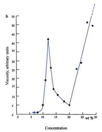
**Fig. 2.30** (a) Phase diagram of poly-*p*-benzamide in tetramethylurea–LiCl solutions. Note that the anisotropic state is obtained under certain conditions [with permission from Magat (1980)] (b) Viscosity vs. polymer concentration in solution. A sharp drop in viscosity occurs when the solution starts becoming anisotropic liquid crystal [after Kwolek and Yang (1993)]
