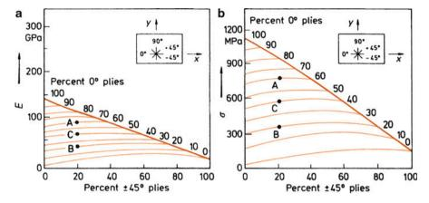
Fig. 14.1 Carpet plots for 65 %  $V_{\rm f}$  carbon/epoxy with a 0°/ $\pm$ 45°/90° stacking sequence: (a) Young's modulus, (b) tensile strength. [From Kliger (1979), used with permission]
