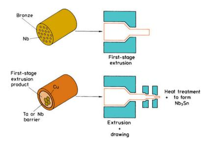
Fig. 9.8 Schematic of the bronze method of fabricating Nb<sub>3</sub>Sn/Cu superconductor
