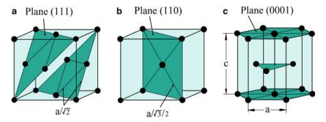
**Fig. 3.13** Three crystalline forms of metals: (a) Face-centered cubic, (b) body-centered cubic, (c) hexagonal close packed. a is the side of the cube in (a) and (b), while it is the side of the hexagon base in (c)
