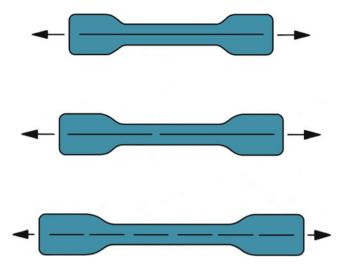
**Fig. 4.12** A single-fiber fragmentation test. On loading the composite, the load is transferred to the fiber and on continued loading it fragments into smaller pieces until the fiber fragment length becomes too small to enable loading it to fracture
