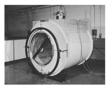
Fig. 9.15 A magnetic resonance imaging system for clinical diagnostics, under preparation (courtesy of Oxford-Airco)
