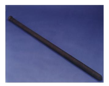
Fig. 7.28 A candle-type filter consisting of Nextel<sup>TM</sup> 312 ceramic fibers in a silicon carbide matrix. The filter is 1.3 m long. Such filters are used to remove particulate matter from high-temperature gas streams up to 1,000  $^{\circ}$ C (courtesy of 3M Co.)
