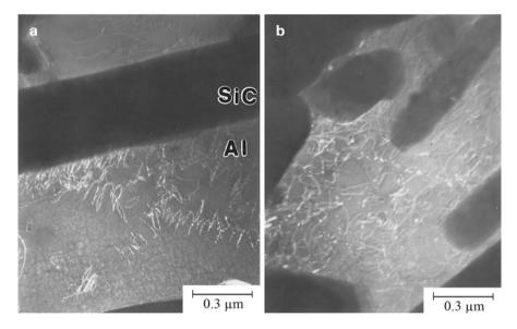
Fig. 6.26 Dislocation distribution in the aluminum matrix of a  $SiC_w/Al$  composite: (a) inhomogeneous dislocation distribution before testing, (b) uniform dislocation distribution after fatigue testing. [From Williams and Fine (1985a), used with permission]
