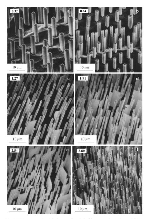
**Fig. 6.9** Transverse sections of in situ composites obtained from a eutectic at different solidification rates indicated in *left-hand top* corners (cm/h). The nickel alloy matrix has been etched away to reveal the TaC fibers. [From Walter (1982), used with permission]
