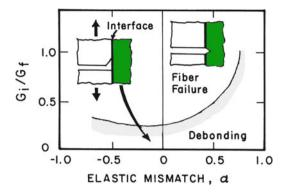
Fig. 7.23 Fiber/matrix debonding criterion in terms of the energy requirements.  $G_i$  is the mixed-mode interfacial fracture energy of the interface,  $G_f$  is the mode I fracture energy of the fiber, and  $\alpha$  is a measure of elastic anisotropy,  $\bar{E} = (E/1 - v^2)$  [after He and Hutchinson (1989)]
