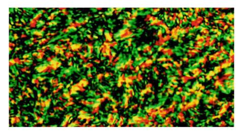
Fig. 2.29 Anisotropic Kevlar aramid and sulfuric acid solution at rest between crossed polarizers [courtesy of Du Pont Co.]
