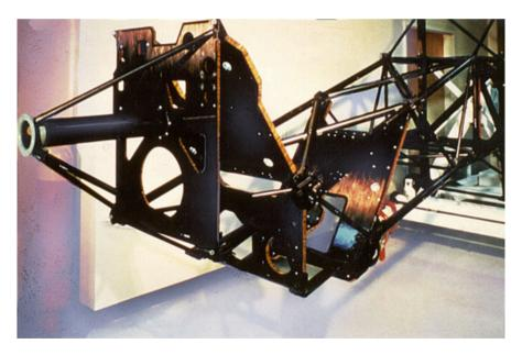
$\textbf{Fig. 5.26} \ \ \textbf{Intelsat 5 has a primary structure and several antennas made of carbon fiber PMCs (courtesy of Fiberite Co.) }$
