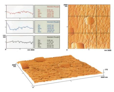
**Fig. 4.3** Characterization of surface roughness of a polycrystalline alumina fiber (Nextel 610) by atomic force microscopy. The three profiles on the *left-hand side* correspond to the two horizontal and one vertical lines on the *right-hand side* figure. The *bottom figure* shows a three-dimensional perspective view of surface
