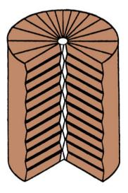
The structure of Kevlar aramid fiber has been investigated by electron microscopy and diffraction. A schematic representation of the supramolecular structure of Kevlar 49 is shown in Fig. 2.35 (Dobb et al. 1980). It shows radially arranged, axially pleated crystalline supramolecular sheets. The molecules form a planar array with interchain hydrogen bonding. The stacked sheets form a crystalline
