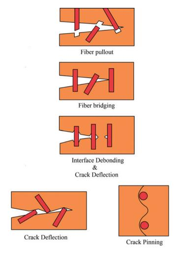
Fig. 7.16 Schematic of some toughness or energy-dissipating mechanisms that can be brought to play in CMCs
