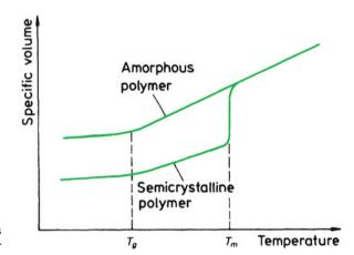
**Fig. 3.2** Specific volume vs. temperature for an amorphous and a semicrystalline polymer
