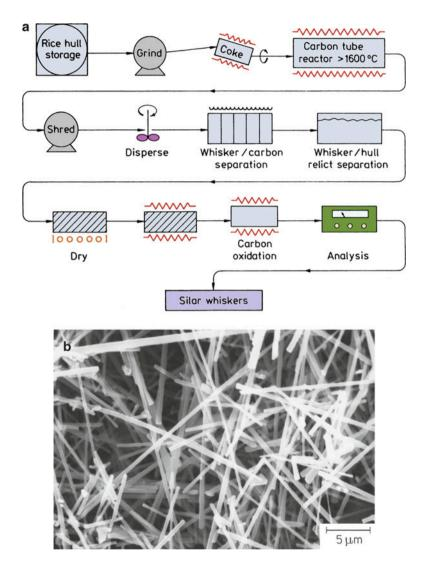
**Fig. 2.45** (a) Schematic of SiC whisker production process starting from rice hulls. (b) Scanning electron micrograph of SiC whiskers obtained from rice hulls [courtesy of Advanced Composite Materials Corporation (formerly Arco)]
