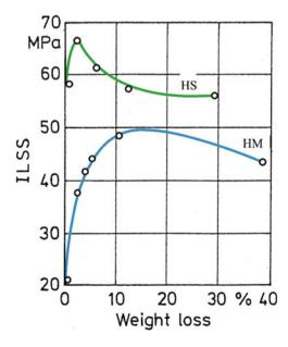
Fig. 5.15 Interlaminar shear strength (ILSS) as a function of weight loss on oxidation. A high-weight loss corresponds to a high degree of oxidation. Note that the maximum ILSS corresponds to less than 10 % weight loss in both cases. [from Clark et al. (1974), used with permission]
