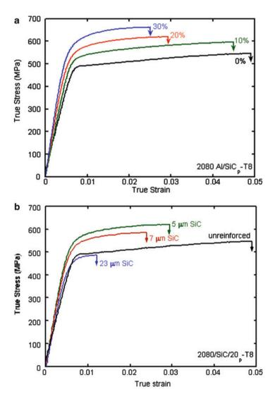
Fig. 6.22 (a) True stress—true strain curves for different volume fractions of the SiC particles in aluminum matrix (6  $\mu$ m). As the particle volume fraction increases, the strength of the composite increases but the ductility decreases. (b) True stress—true strain curves for different particle sizes but for a fixed volume fraction (20 % by volume). The strength increases as the particle size decreases. [Courtesy of N. Chawla]
