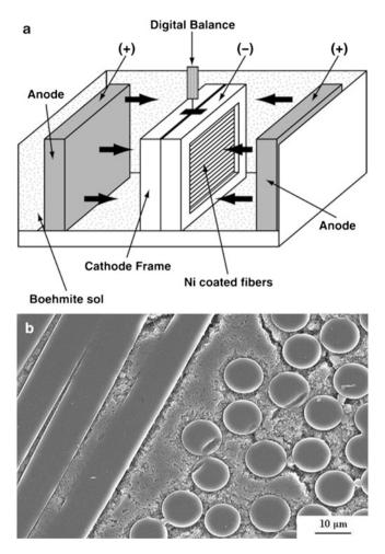
**Fig. 7.10** (a) Schematic of the basic electrophoretic deposition (EPD) cell. (b) Microstructure of Nicalon 720 fiber/mullite composite made by electrophoretic deposition (from Kaya et al. 2009)
