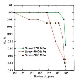
Fig. 13.9 Typical modulus loss curve for unidirectional silicon carbide/aluminum composites.  $E_N$  is the modulus after N cycles and  $E_0$  is the modulus in the uncycled state [after Gomez and Wawner (1988)]
