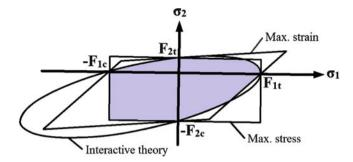
Fig. 12.15 Failure envelopes due to different failure criteria. The *shaded part* indicates the conservative failure region [after Daniel and Ishai (1994)]
