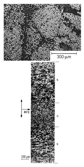
**Fig. 5.16** (a) Continuous glass fibers in a polyester matrix showing resin-rich regions. (b) Discontinuous glass fibers in a semicrystalline polyethylene terephthalate thermoplastic matrix showing anisotropic distribution of fibers. MFD denotes the mold fill direction. S and C denote the surface and central layers, respectively [from Friedrich (1985), used with permission]
