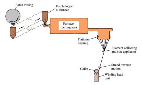
Fig. 2.3 Schematic of glass fiber manufacture
