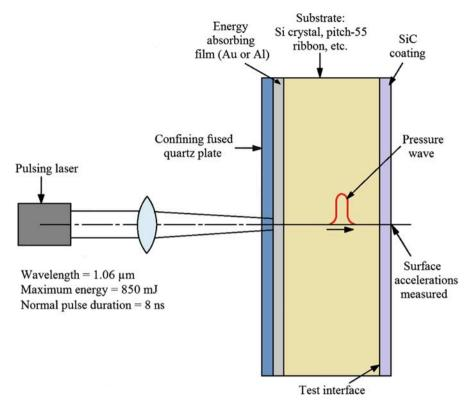
**Fig. 4.13** Experimental setup for a laser spallation test. A collimated laser pulse impinges on a thin film sandwiched between the substrate and a confining plate. Absorption of the laser energy in the constrained aluminum film causes a sudden expansion of the film, which produces a compressive shock wave in the substrate that moves toward the coating/substrate interface. This compressive pulse is reflected into a tensile pulse at the free surface of the coating
