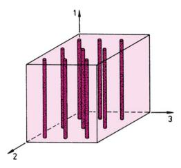
Fig. 10.4 A transversely isotropic fiber composite: plane transverse to fibers (2–3 plane) is isotropic
