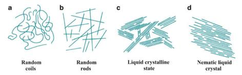
**Fig. 2.28** Various states of polymer in solution: (a) two-dimensional, linear, flexible chains (random coils), (b) random array of rods, (c) partially ordered liquid crystalline state, and (d) nematic liquid crystal (randomly distributed parallel rods)
