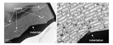
$\textbf{Fig. 15.6} \quad \text{Deformation of SiC/Al nanolaminate in a nanoindenter. Note the well-bonded interface and the extreme flexibility of SiC, an inherently brittle material } \\$
