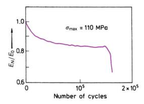
Fig. 13.12 Stiffness reduction curve for a  $[0^{\circ}/90^{\circ}]_s$  glass fiber reinforced laminated composite [after Ogin et al. (1985)]
