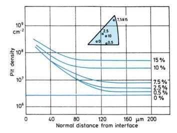
Fig. 10.10 Variation of dislocation density ( $\simeq$ pit density) with distance from the interface. The higher dislocation density in the plateau region with high  $V_f$  is due to a higher  $\sigma_z$  with higher  $V_f$  (Fig. 10.9) [from Chawla and Metzger (1972), used with permission]
