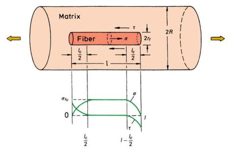
Fig. 10.15 Load transfer in a fiber/matrix composite and variation of tensile stress ( $\sigma_f$ ) in the fiber and interfacial shear stress ( $\tau$ ) with distance along the interface
