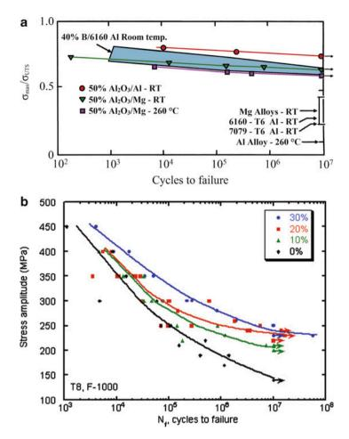
**Fig. 13.5** (a) *S–N* curves for MMCs in tension–tension for unidirectionally reinforced boron fiber (40 % v/o)/A16061, alumina fiber (50 % v/o)/Al, and alumina fiber (50 % v/o)/Mg composites [after Champion et al. (1978)]. (b) *S–N* curves for silicon carbide particle reinforced aluminum matrix composites [courtesy of N. Chawla]
