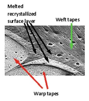
Fig. 15.3 Microstructure of a self-reinforced composite (PP fabric in a PP matrix)
