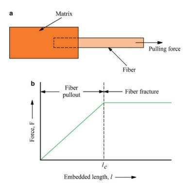
Fig. 4.8 (a) An experimental setup for a single fiber pullout test. A portion of fiber, length l, is embedded in a matrix and a pulling tensile force is applied as shown. (b) The stress required to pull the fiber out of the matrix as a function of the embedded fiber length
