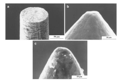
Fig. 4.9 Three different types of indenters: (a) cylindrical with a flat end, (b) conical with a flat end, and (c) pointed (courtesy of J. Janczak-Rusch and L. Rohr)
