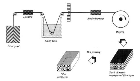
Fig. 7.1 Schematic of the slurry impregnation process
