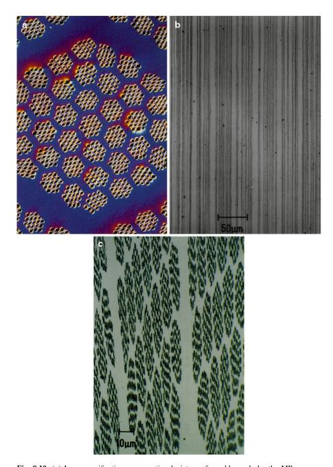
**Fig. 9.10** (a) Low-magnification cross-sectional picture of a cable made by the MP process. (b) Longitudinal section and (c) transverse section. The superconductor is  $Y_{0.9}$  Ca $_{0.1}$  Ba $_{2}$  Cu $_{4}$  Ag $_{0.65}$  metallic precursor/silver composite containing 962,407 filaments (courtesy of American Superconductor Co.)
