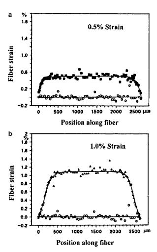
Fig. 10.16 Micro-Raman spectra of Kevlar aramid 149 when the Kevlar/epoxy composite is loaded axially. (a, b) Strain build up in the fiber from the two ends. (c, d) Fiber fracture leads to a drop in strain at those sites [after Young (1994)]
