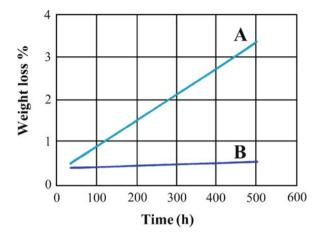
**Fig. 2.25** Oxidation resistance, measured as weight loss in air at 350 °C, of carbon fibers having different moduli: (*A*) Low modulus Celion 3000 (240 GPa) and (*B*) High modulus Celion G-50 (345 GPa) [after Riggs JP (1985) Encyclopedia of polymer science and engineering, 2e, vol 2, John Wiley and Sons, New York, reprinted with permission]
