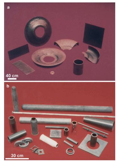
**Fig. 7.5** Some fiber reinforced ceramic components made by Dimox process. (a) Fiber reinforced ceramic composites for applications in high-temperature gas turbine engine components. (b) Heat exchanger and radiant burner tubes, flame tubes, and other high-temperature furnace parts made of particle reinforced ceramic composites. (Courtesy of Lanxide Corp.)
