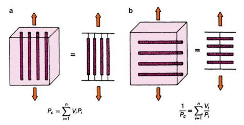
Fig. 10.1 Unidirectional composite: (a) isostrain or action in parallel and (b) isostress or action in series
