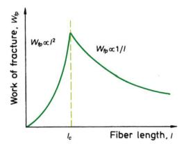
Fig. 12.5 Variation of work done in fiber pullout with fiber length
