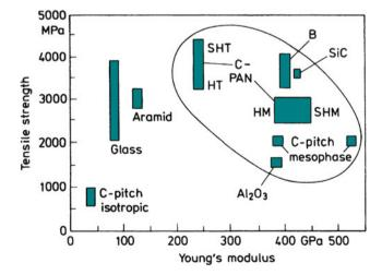
Fig. 2.47 Comparison of different fibers
