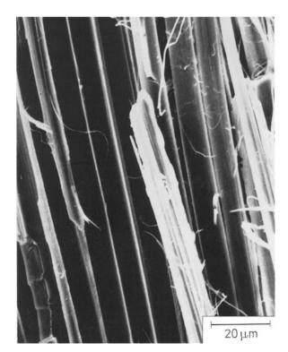
Fig. 12.6 A delaminationtype fracture of Kevlar/epoxy composite. Note the characteristic fibrils in the fiber [from Saghizadeh and Dharan (1985), used with permission]
