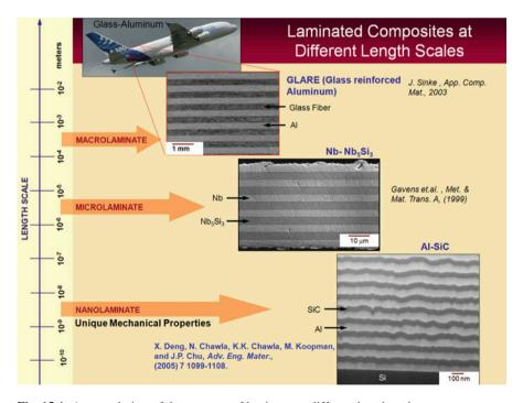
Fig. 15.4 A general view of the structure of laminates at different length scales
