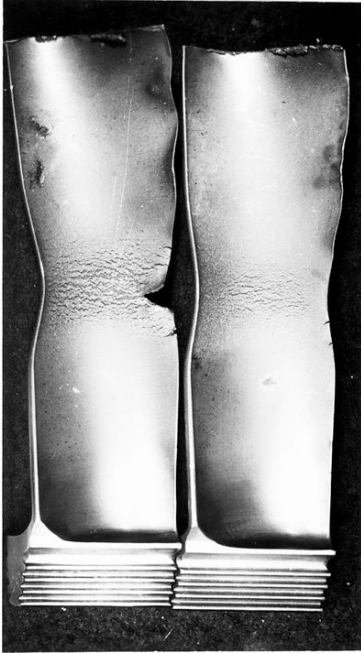
(a) Turbine blades with large creep deformation and cracking due to overheating. Blade length 11 cm
