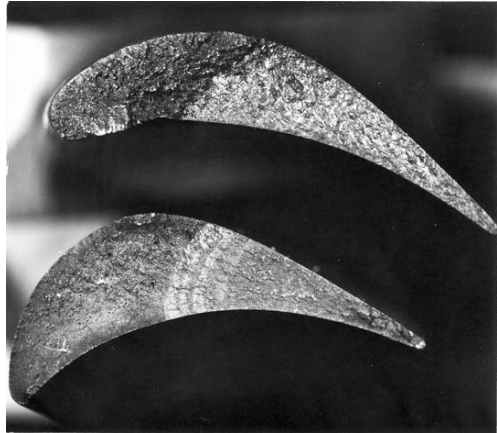
(b) Fatigue failures in turbine blades starting at the trailing edge (blade chord 25 mm)
