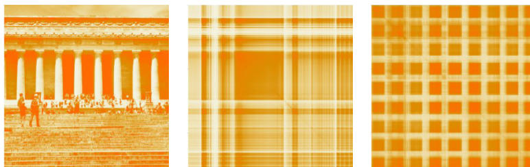
Figure 8.5: The Lincoln memorial M (left) and its covariance matrices. The big block in the middle of M \cdot M^T (center) results from the similarity of all rows from the middle stripe of M . The tight grid pattern of M^T \cdot M (right) reflects the regular pattern of the columns on the memorial building.
