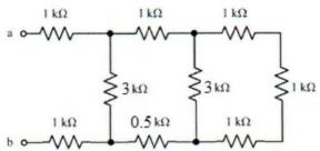
ii. Evaluate the equivalent resistance (RAB) of the following infinite network of resistance. (5 marks)
