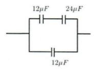
c) Find the charge on each of the capacitors in the figure below.
