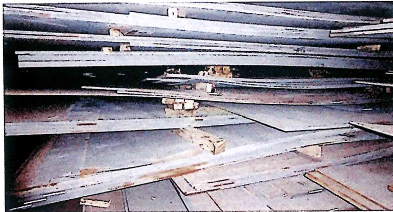
✘ Improper stow, alignment and use of dunnage
