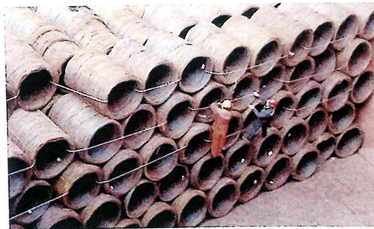
✘ Lashing the vertical face. Note the lack of safety harnesses. No safety access to the vertical part of the stow
