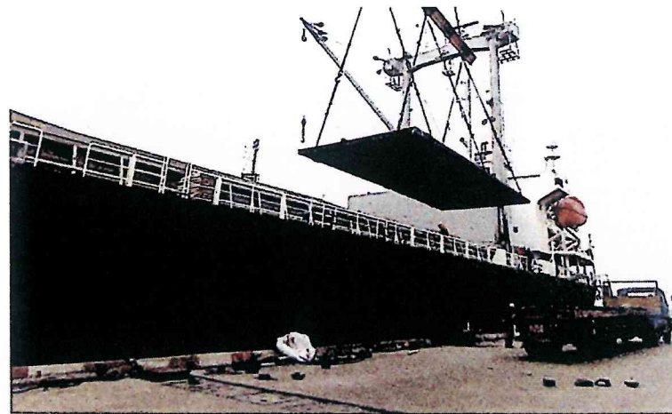
✔ Discharging of unbundled, unpacked steel plates
