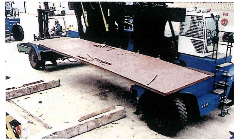
✔ Jurong Port is equipped with side-loaders with an SWL of 22 tonnes each
