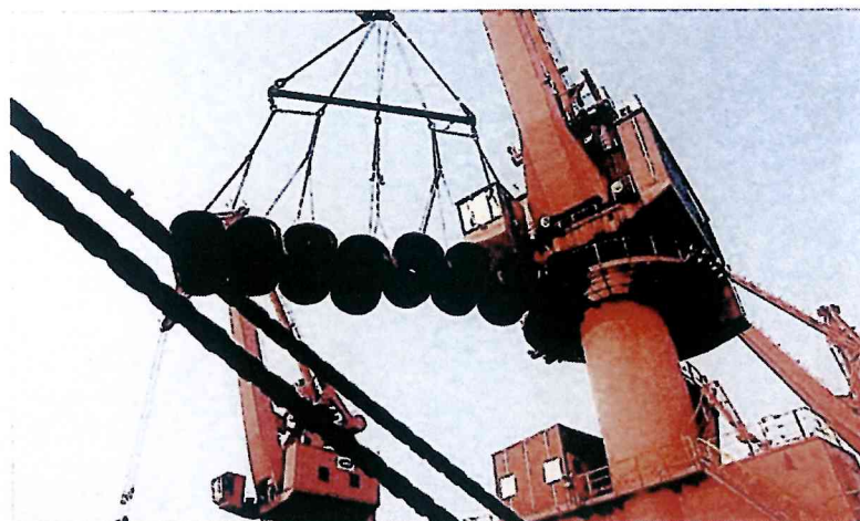
✗ In this set-up, eight coils are loaded. However, the slings are made of wire. This is not recommended as it may damage the coils or their securing straps/wires
