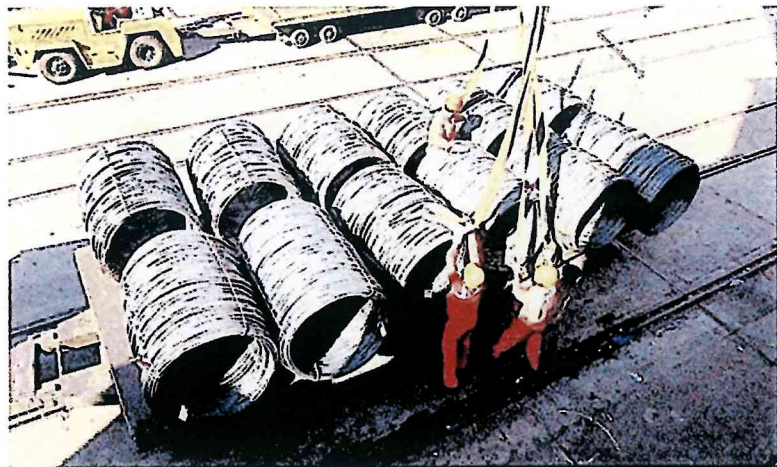
✓ Slings the coils for loading. One nylon belt per coil is used to avoid damage to the cargo
