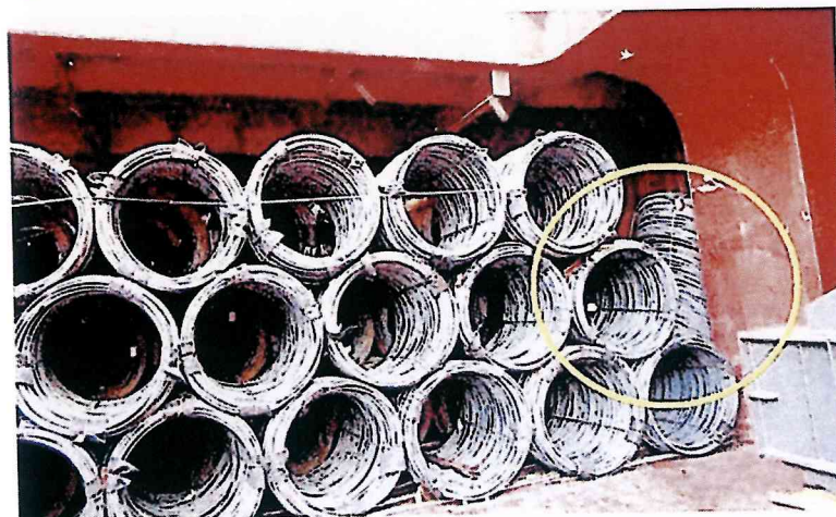
❌ One coil has fallen off the stow and is sitting vertically and unsecured
