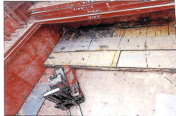
✔ Use of a forklift truck for the discharging of steel plates in a hopper-type cargo hold. Handling of steel plates underneath the coamings
