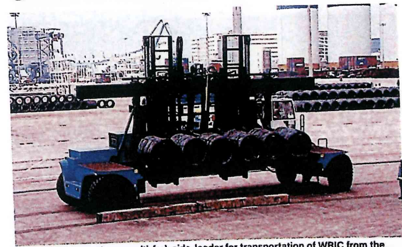
✓ Jurong Port has a multi-fork side-loader for transportation of WRIC from the quay to the storage area
