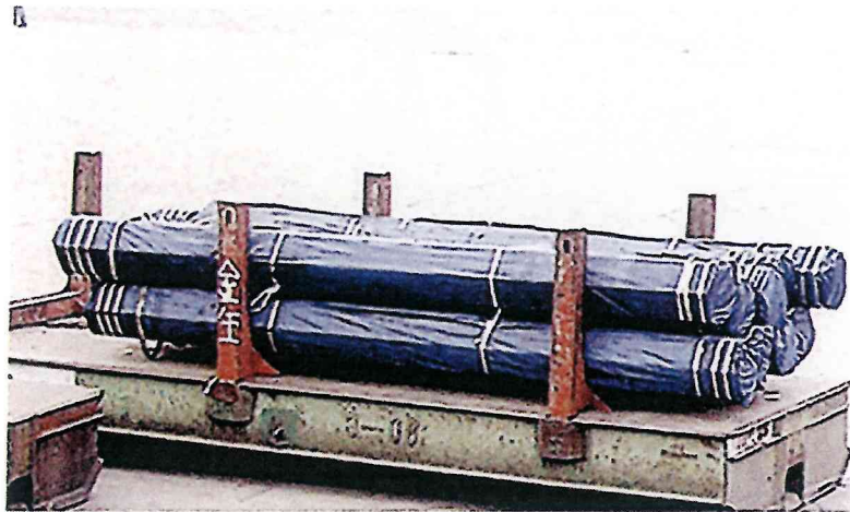
✓ Pre-slung bundled and packaged pipes on the quay prior to loading Note: the pre-slings are for tip-lifting only
