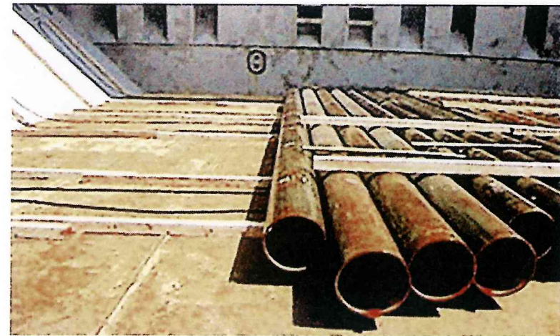
✓ Dunnage laid on the tank-top and on subsequent layers of medium-size pipes
