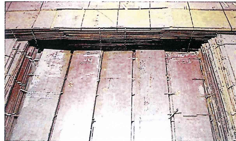
✓ Stow of steel plates in longitudinal and athwartships direction. The upper tiers only are lashed with steel bands
