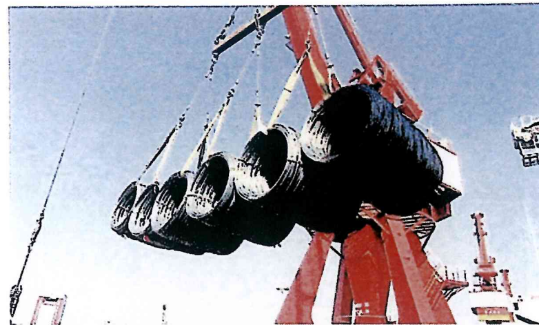
✓ By using lifting strops attached to beams (spreader), up to six coils at a time may be loaded in this layout
