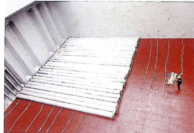
Dunnage being laid on the tank-top in preparation for the loading of loose pipe
