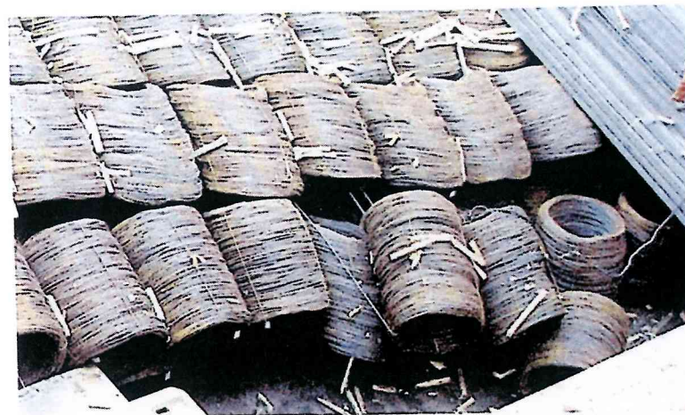
✘ Collapsed stow and deformed coils due to loading cargo above the coils
