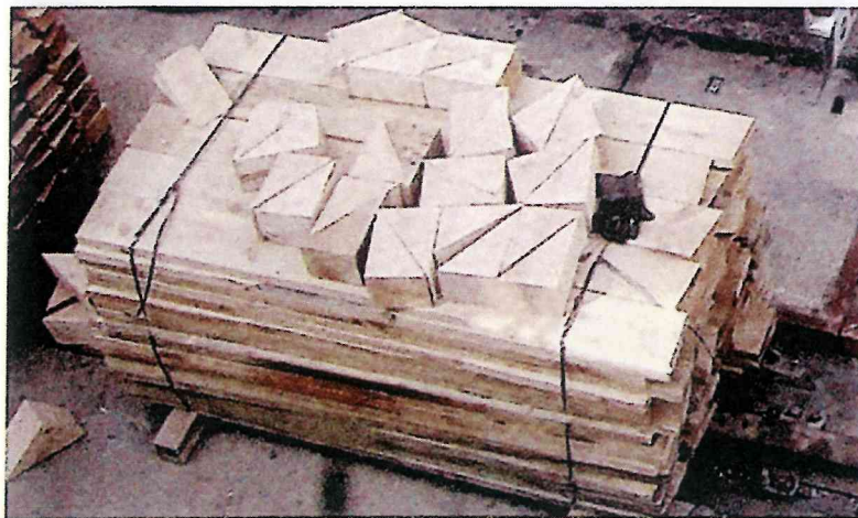
✓ Good-quality soft wood dunnage boards and wedges to be used on the tank-top or hatch cover. Ideally, the boards should be of 150 mm x 25 mm cross-section
