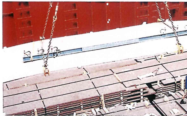
✓ Good storage and use of dunnage for steel plates
