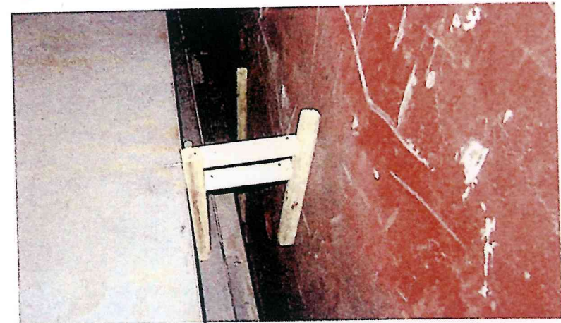
✗ A single chocking of the last two tiers must not be done this way. The dunnage in the photograph is not sufficient and may slip. The chocking should be along the length of the bulkhead
