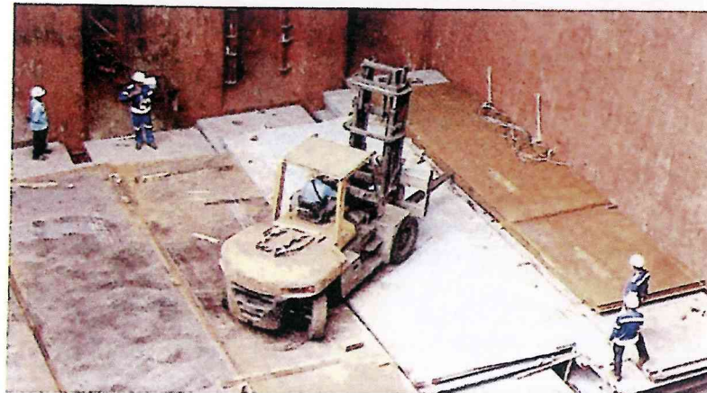
✗ The fork is used to separate the plates and create space for placing dunnage before the final lift is done with the truck
