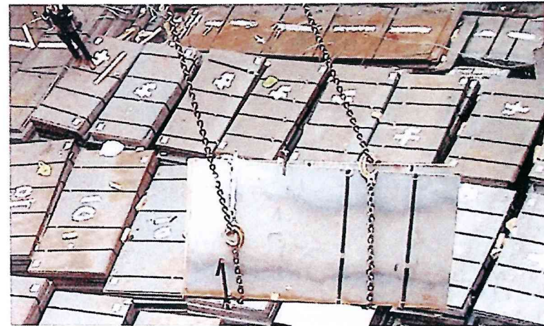
✗ Bundled steel plates. Broken steel straps. Incorrect choke hitch application
