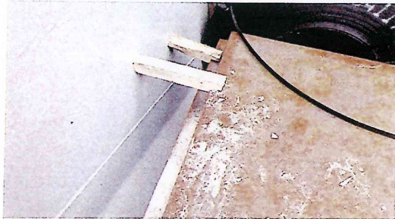
✘ Incorrect use and securing of dunnage. The wood may easily slip from the bulkhead and fall from its place during voyage
