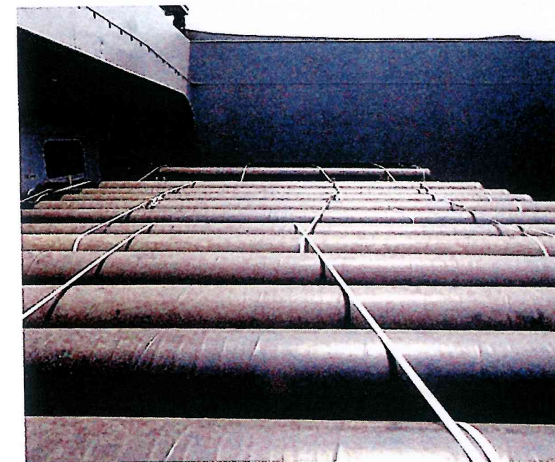
Nylon web strapping used to lash a stow of medium-size pipes. The lashing is made only on the top tier of pipes in a box-shaped cargo compartment
