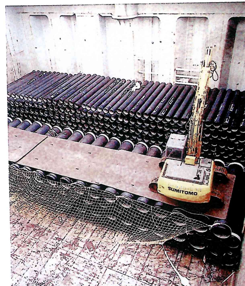
Two uniform stows of pipes. Note that the swaged ends are stowed at opposite ends on alternate layers and the faces are stepped accordingly
