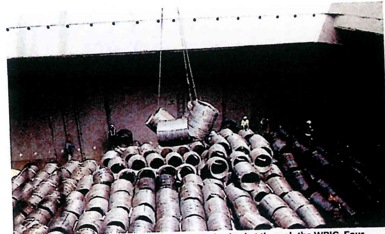
✓ The coils will be discharged by a single leg basket through the WRIC. Four WRIC handled with two wire slings
